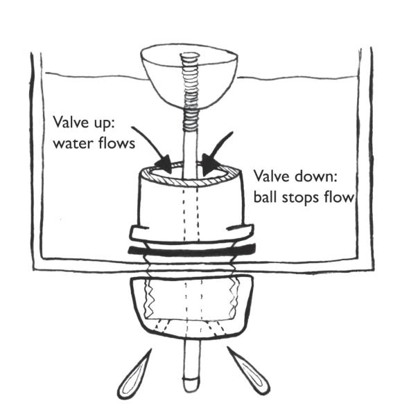
A tap of the hand pushes the rod up, opens the valve and allows a small amount of water to flow.
