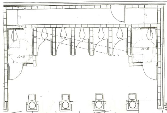
Drawings by restroom design consultant Mary Coakley for PHLUSH. Note roofless open plans, direct access stalls & external wash basins.
